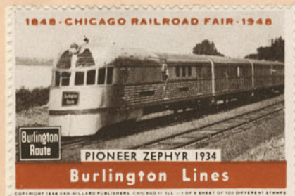
America's first Diesel-powered streamlined train was introduced by the Burlington in 1934. That year it ran 1015 miles non-stop Chicago to Denver, averaging 77.6 m.p.h.
