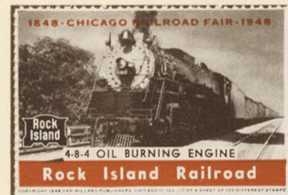
An example of locomotive development is this oil-burning steam engine with 4-8-4 wheel arrangement; overall length with tender, 108 feet, 10 inches.
