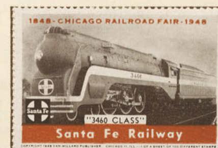
The Santa Fe, 3460 series, is of the 4-6-4 type, an improved Pacific type.
