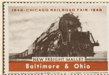
Giant Mallet locomotives—pride of Baltimore & Ohio's freight fleet—can each move 15,000 tons at an average speed of 30 miles an hour.
