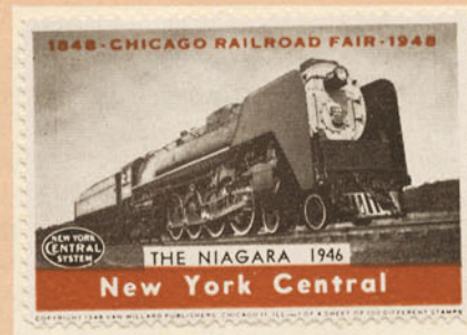
The Niagara, built in 1946, is a giant 4-8-4, double duty freight and passenger locomotive.
