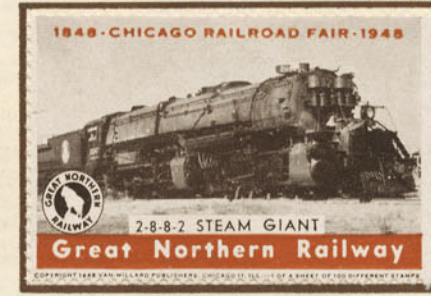
Moving Great Northern freight trains is this giant articulated steam locomotive with 2-8-8-2 wheels. Over-all length is 120 feet.
