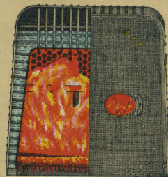
Cross Section. End Elevation. View Showing Boiler Cut Half-way Across Through Fire-box.
