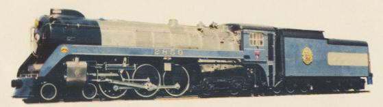
Locomotive Nos.2850 to 2859. Class—H-1-d. Cylinders—22 inches diameter by 30-inch stroke. Drivers—75 inches diameter. (Six) Boiler Pressure—275 pounds per square inch. Tractive Power—45,250 pounds. Tractive Power with Booster—57,250 pounds.
