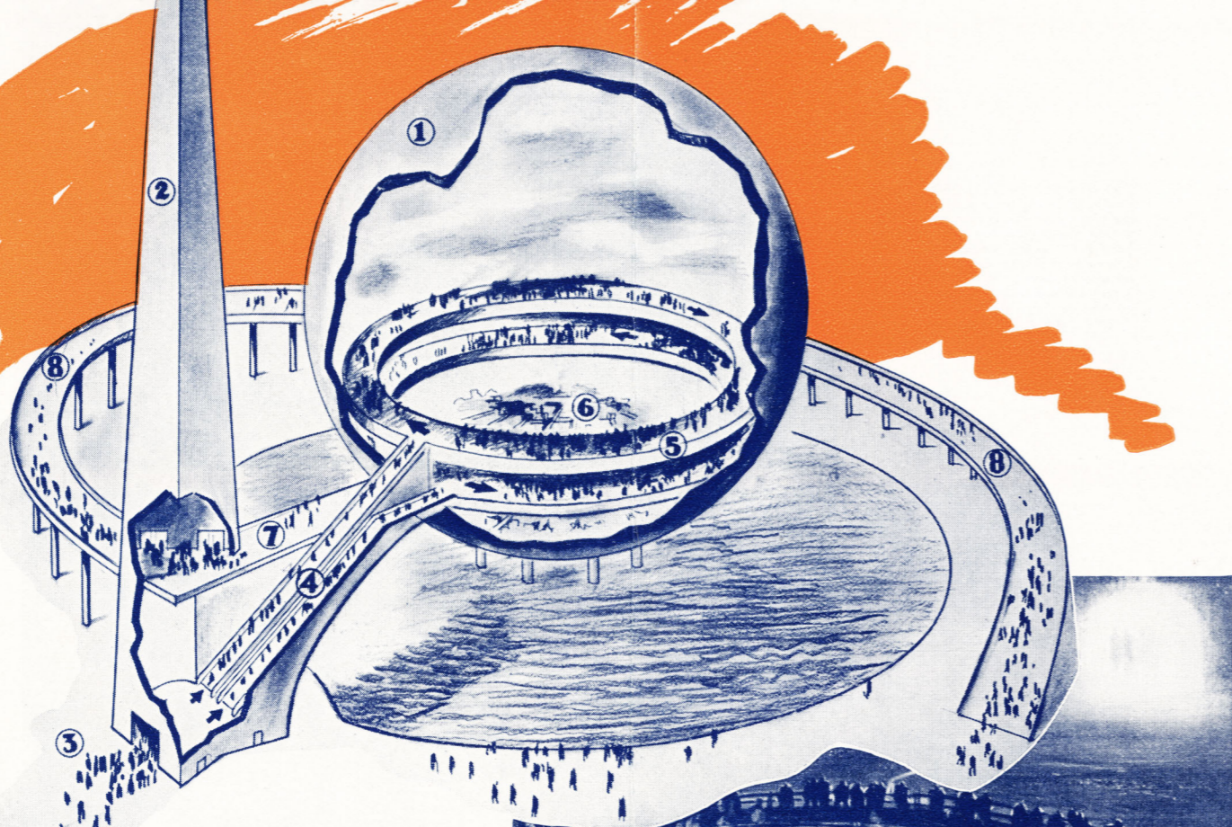
Cut-away drawing shows the Theme Center of the New York World's Fair 1939. This unique twin structure will house the focal exhibit of the Exposition. The drawing shows: 1—Perisphere, a 200-ft. sphere. 2—Trylon, a 700-ft. triangular obelisk. 3—Entrance to exhibit. 4—Escalators carrying visitors to 65-ft. level. 5—Revolving platform from which to view the interior. 6—Model of the City of Tomorrow. 7—Exit Bridge leading to descending ramp. 8—Helicline or Exit Ramp encircling the structures.
