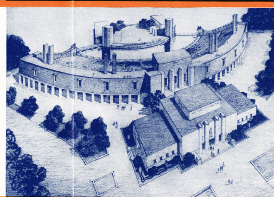
New York State Exhibit Building and Fountain Lake Amphitheatre on Fountain Lake in the Fair's Amusement Area, from an artist's sketch of the $2,200,000 project. The stage will be 60 feet offshore; the seating capacity of this permanent structure will be 10,000. Exhibit building in foreground will be temporary for the Fair period.
