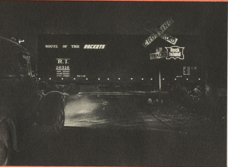
NEW "SAFETY SIGNS" —Even that commonplace workhorse of the railroad, the boxcar, gets a new look! Special reflecting material applied to the cars picks up headlight beams from your auto, can be seen for considerable distance—another measure adding to the safety of grade crossings.
