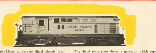
The Fairbanks-Morse all-purpose diesel electric loco-motive is an 0.4.4.0 type of 1500 HP, a number of which have recently been placed in service of Union Pacific. This type is also known as a "road-switcher" since it
