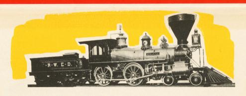
Locomotive No. 22 was built in 1875 by Baldwin Locomotive Works and was known as an "eight-wheeler". The drive wheels are 57 inches in diameter and it operates with a boiler pressure of 130 pounds. This speedy woodburner of yesteryear stands 14 feet
