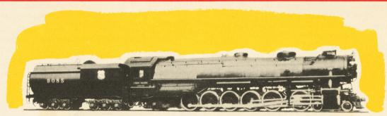
The 9000 class, 4-12-2 type locomotive is known as the "Union Pacific" because it was designed by the Engineering Department of the Union Pacific Railroad at Omaha. It was first placed in service in 1926 and has remained a mainstay of steam motive power on the railroad for over two decades.
