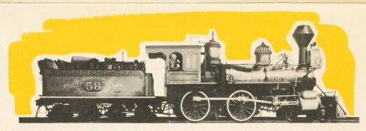
Constructed in 1874, the old time woodburner No. 18 was the pride of its railroading day. Known as an "eight-wheeler", the 60-inch main driving wheels mark it as a fast passenger locomotive and it operates with 130 pound boiler pressure. No. 18 is the same as No. 58 shown above.
