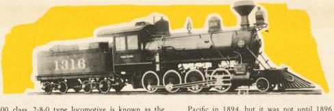
The 400 class, 2-8-0 type locomotive is known as the "Consolidation" type. Type 2-8-0 stands for the wheel arrangement under the locomotive, that is, there are two forward truck wheels, eight driving wheels, and no trailing truck wheels on this locomotive. This designation is used universally in the United States to dis-
