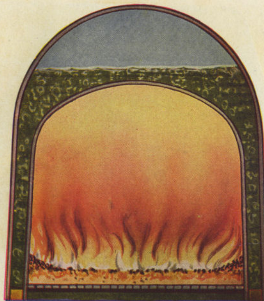
Plate 1. PERFECT CONDITION of Fire Bed—CROSSWISE. Level throughout the MIDDLE—but thicker along the SIDES—because the Draft acts stronger and requires more fuel there than in the central part. See subject 43.
