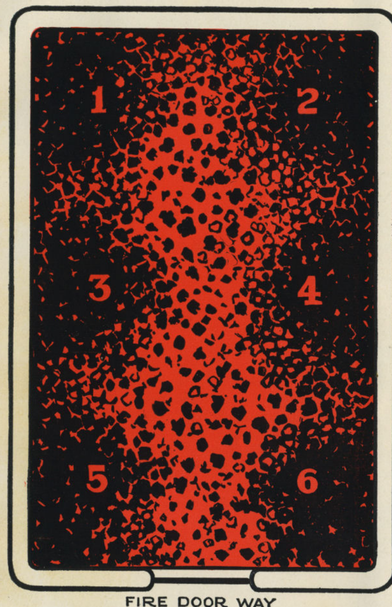
FIG 4. DIAGRAM SHOWING PLAN OF CROSS FIRING.
