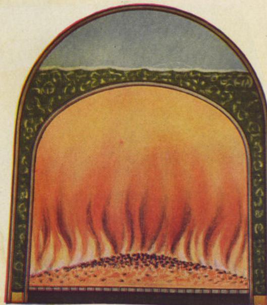
Plate 2. WRONG CONDITION of Fire Bed. Too deep in the MIDDLE—where the Draft is weakest—and too shallow at the Sides where the Draft is strongest. Compare Plates 1 and 2.
