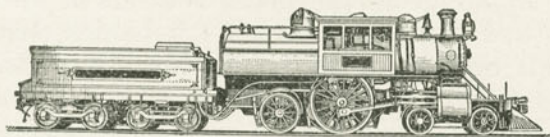
Baldwin Single Driver Passenger Locomotive, capable of great speed. Diameter of cylinders, high pressure, 13 inches, low pressure, 22 inches; stroke, 26 inches; diameter of driving wheels, 84 \frac{1}{4} inches; total wheel base, 22 feet, 9 inches; weight on drivers, 48,000 pounds; total weight of locomotive, 115,000 pounds.
