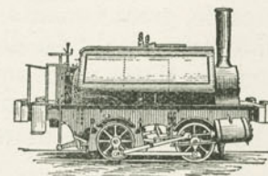
Scotch Tank Engine, for light switching purposes. Diameter of cylinders, 8 in.; stroke, 18 in.; diameter of driving wheels, 2 ft., 6 in.; fixed wheel base, 5 ft.; tank capacity, 220 gals.; fuel space, 11 cu. ft.; weight of locomotive, 17,580 lbs.
