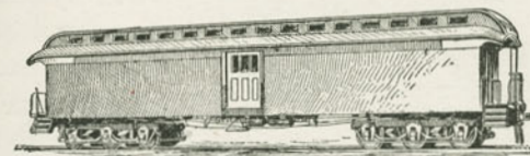
Standard American Baggage Car. Length, 50 ft.; height above the rail, 14 ft.; weight, 52,350 lbs. A portion of the car is frequently set aside for the express or parcel traffic. The mail also is frequently carried in this car on irregular trains where the business is not sufficient to warrant a messenger. In the early history of railways the baggagemen handled all the mail matter which railways carried.
