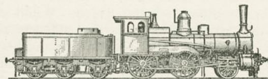
German Rapid Transit Passenger Locomotive, with Belpaire type of fire box, Warschau-Wien Railroad. Diameter of cylinders, 17 in.; stroke, 22 in.; diameter of driving wheels, 72 in.; weight of locomotive, 73,719 lbs.; water capacity of tender, 2,614.7 gals.; coal capacity, 8,828 lbs.; weight of tender, loaded, 59,500 lbs.
