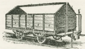
Italian Half Box Car. Length, 14 ft., 9 in.; height of sides, 36 in.; weight, 3 tons; load, 8 tons. This car, while supplied with a ridge pole, has no roof. It thus becomes what is known in the United States as a gondola car, and in other countries as a half box car.
