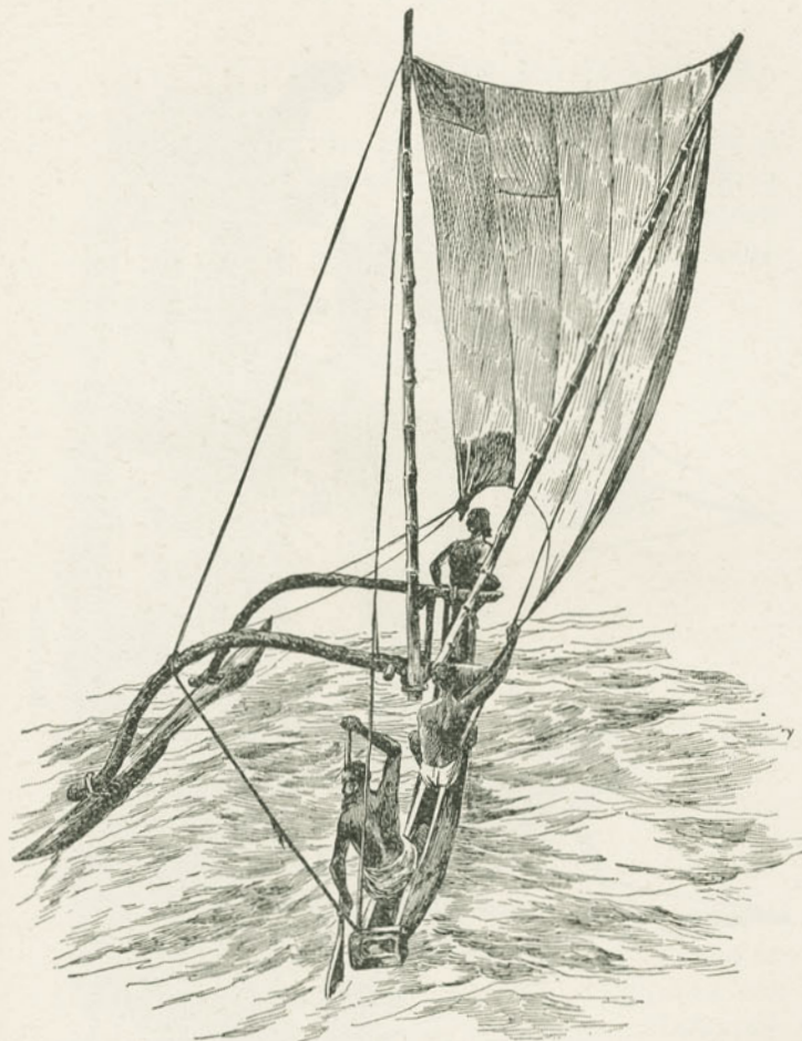
Singalese fishermen off the coast. When the outrigger is not heavy enough to hold the boat down, the weight of one or more of the crew is added to it.
