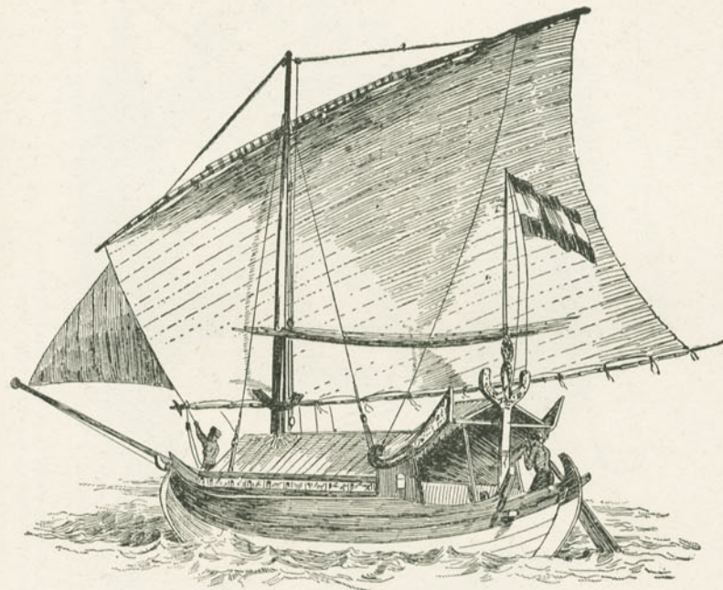
Off the coast of Java. It is said that the method of rigging sailing vessels in the classical period was the same as the above, namely, one mast with two yards and a square sail.
