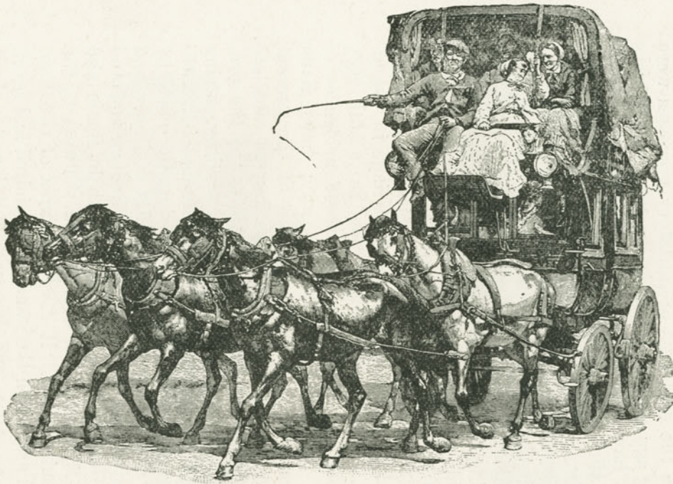
A French diligence in the Pyrenees mountains. These vehicles consist of three compartments: the front, called the coupe , for three persons; the second, called the interieur , for six persons; and the rotonde , entered from the rear, for six persons. Above in front is the banquette , where the conductor is seated, and behind this, underneath a thick leather covering, passengers are sometimes huddled among the baggage.
