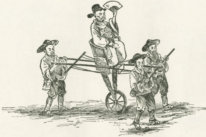
A Korean monocycle or chair. The weight of the passenger is borne by the wheel, which is kept erect by the coolies.
