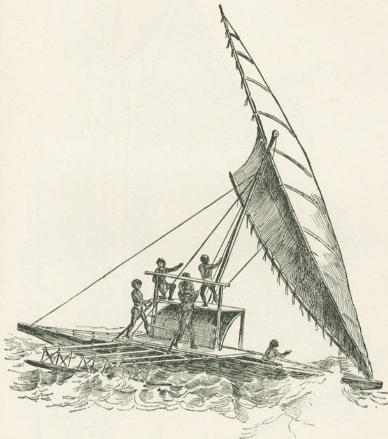
A characteristic Malay craft. The outrigger steadies the vessel, it will be noticed, and thus permits a great spread of canvas.
