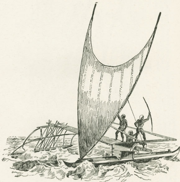
A primitive war vessel. The arm of the outrigger is used to carry the warriors and at the same time trim the vessel. The sail is made of skins fastened to bamboo poles. The end of the sail resting on the stern of the boat is held in place by guy ropes from the sides.
