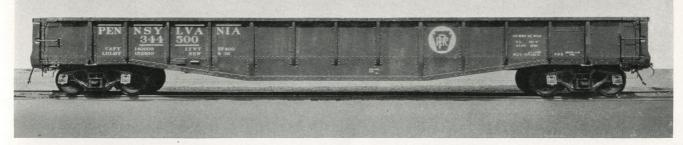
MILL TYPE GONDOLA CAR All steel. Drop ends. For pipe, structural shapes, etc.
