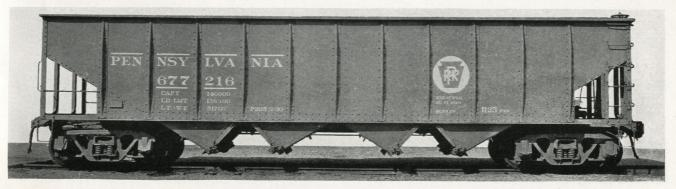
HOPPER CAR All steel. For coal, ore and other heavy bulk commodities.
